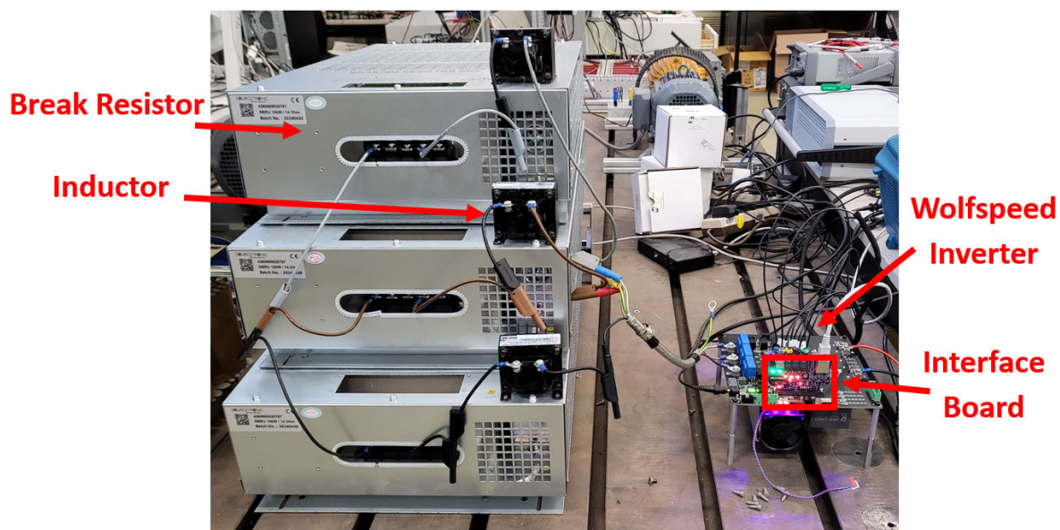
Figure 4.11: Integrated testing setup with resistors and inductors
